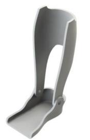
Fig. 3. The CAD model of the active orthoses realized in Solidworks 2016
