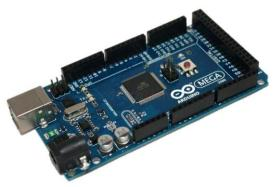
Fig. 5. Arduino Mega 2560 [4]
