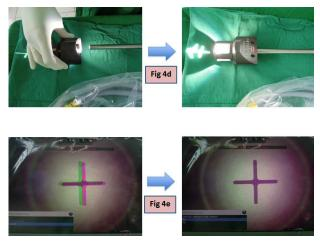
Fig 4d-4e. Endoscope alignment target for 3D calibration
