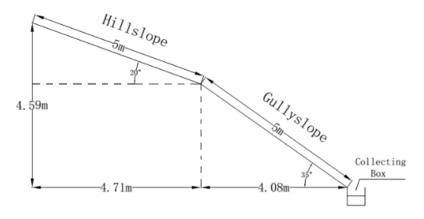
Fig.1 Sketch map of experimental soil bed of slope-gully system
