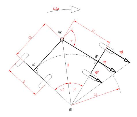
Fig. 3 Curved travel, horizontal projection O1 – instantaneous centre of the wheel loader rotation; SP – centre of the front axle; SZ – centre of the rear axle; VK – vertical hinge; L1, L2 – distances of axles from the vertical hinge; B – wheel track;  $R_z$  – instantaneous turning radius;  $\omega_z$  – angular speed relating to the centre of rotation
