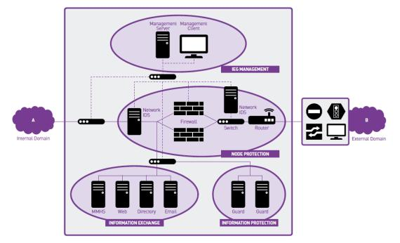
Figure 3. The technical interconnection between two systems using IEG's (the picture is taken from the paper "Information Exchange Gateways: Reference Architecture" Nexor, 2009)
