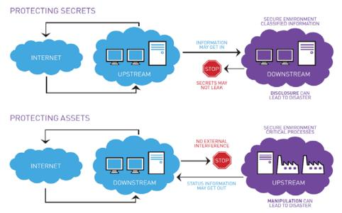
Figure 5. The way the information and physical goods are protected via diodes (images are taken from the paper "Protecting confidential information on Using diodes", Nexor, 2015)
