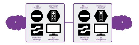
Figure 2. The block diagram interconnection through two IEG's (the picture is taken from the paper "Information Exchange Gateways: Reference Architecture" Nexor, 2009)
