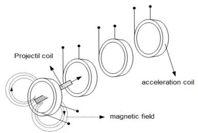
Fig. 1 The operating principle of the electromagnetic coil gun
