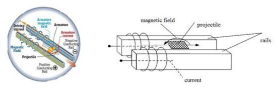
Fig. 3 The operating principle of electromagnetic rail gun
