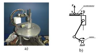
Figure. 8. A test-bed slider-crank mechanism at LARM: a) an experimental set up with accelerometer and weight on the slider. b) sensing axes of the accelerometer.
