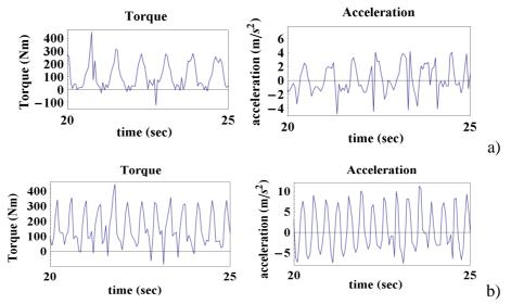
Figure 14. A measure of slider crank with servo motor with earthquake effect (type 1), torque data of the motor, acceleration of the slider with crank rotation: a) 90 rpm, b) 180 rpm
