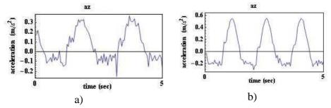
*Figure 9. An experimental measure of the typical acc. of the slider-crank with stationary frame: a) crank rotation 32 rpm, b) crank rotation 43 rpm,*
