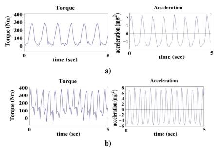
Figure 11. An experimental measure of slider crank with servo motor without earthquake effect: a) torque data of the motor, acceleration of the slider with crank rotation 90 rpm, b) torque data of the motor, acceleration of the slider with crank rotation 180rpm
