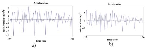
Figure 12. An experimental measure of the typical accelerations with horizontal slider under earthquake effect (type 1): a) crank rotation 32 rpm, b) crank rotation 43 rpm.
