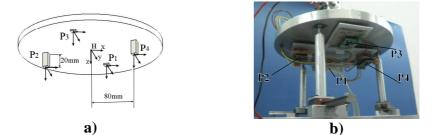
Figure 4. Sensored CaPaMan platform with accelerometers: a) a scheme, b) sensor installation & test lay-out
