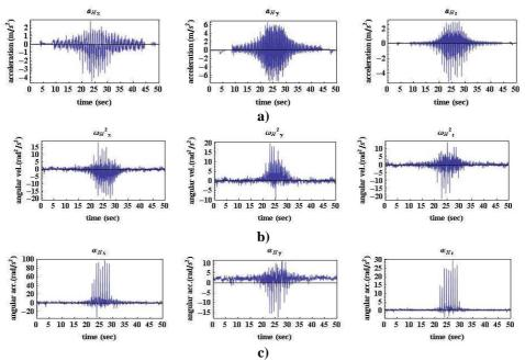
*Figure 7. An example of acc. data during earthquake simulation: a) for platform center H, b) angular platform velocity, c) angular platform acc.*
