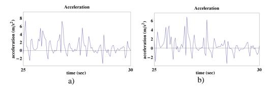
Figure 13. An experimental measure of the typical accelerations with vertical slider under earthquake effect (type 1): a) crank rotation 32 rpm, b) crank rotation 43 rpm.
