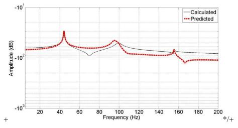
**Figure 4.** Vibration response,  $x_3$  (without considering  $f_3 = 20$  N)
