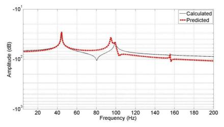
**Figure 3.** Vibration response,  $x_3$  (without considering  $f_3 = 10$  N)
