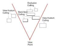
Figure 2. Types of visibility culling methods. A polygon is determined as invisible if it faces away from the viewpoint (Back-Face Culling), is occluded by another part of the scene (Occlusion Culling), or is outside the current viewing frustum (View-Frustum Culling).
