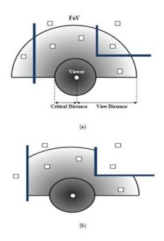
Figure 8. (a) In A3 algorithm, critical distance and view distance are identified. Primitives in the critical area have more priority than others which exist in rest of the FoV. (b) In EA3, only difference from A3 is taking the obstacles into consideration and thus reducing the area of FoV.
