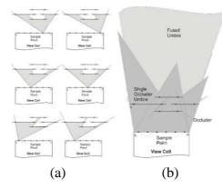
Figure 3. (a) Sampling of the occlusion from six sampling points. (b) The fused umbra from the six points is the intersection of the individual umbra.
