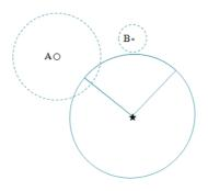
Figure 6. In CyberWalk, since the user's view scope (straight line) overlaps with object A's object scope (dashed line), A is handled for further resolution determination. Though B is closer than A to the user, it is not handled because most probably B's size is much smaller.
