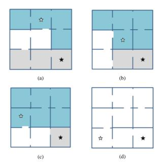
Figure 7. A client pair negotiate and define their frontiers in initial position (a). When at least one of them leave its frontier, they renegotiate and define new frontier regions (b and c). If there is a line of sight between cells those contain client pair, frontier cannot be constructed (d).
