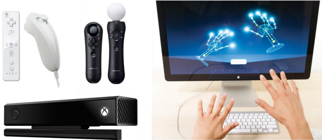
Figure 1. Emerging generation of gesture recognition technology, including the Nintendo Wii, the Sony Playstation Move, the Microsoft Xbox Kinect and the Leap Motion Controller
