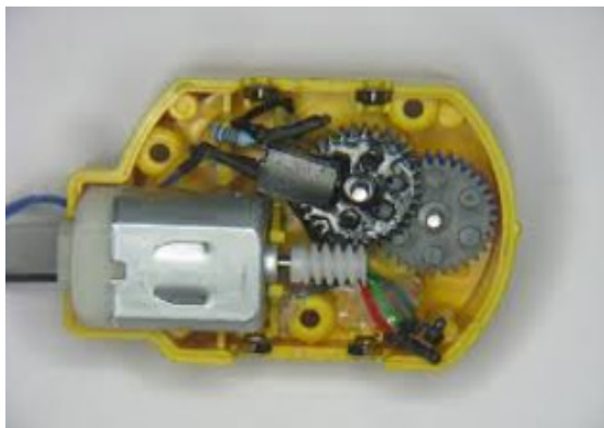
Figure 4. DC motor and gear structure used in the joint of the robot
