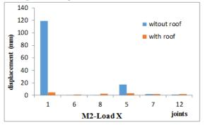
a) X direction displacements of 1-6-8 and 5-7-12 nodes
