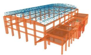
Figure 2. Model M1 (Vault system- 48m\* 40.1 m in plan, h=7 m).
