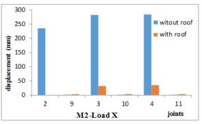
b) X direction displacements of 2-9, 3-10 and 4-11 nodes
