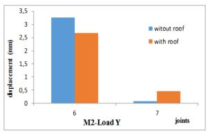
d) Y direction displacements of 6-7 nodes
