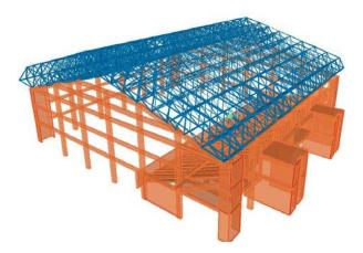
Figure 3. Model M2 (Broken system- 44.7m\*51.2m in plan, h=11 m)
