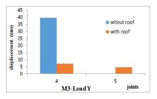
d) Y direction displacements of 4-5 nodes
