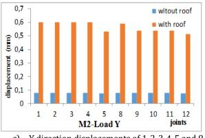
c) Y direction displacements of 1-2-3-4-5 and 8-9-10-11-12 nodes
