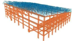
Figure 4. Model M3 (Flat system- 62.5m\*45.2m in plan, h=10 m)
