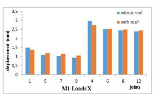
b) X direction displacements of 1-5-7-9 and 4-6-8-12 nodes
