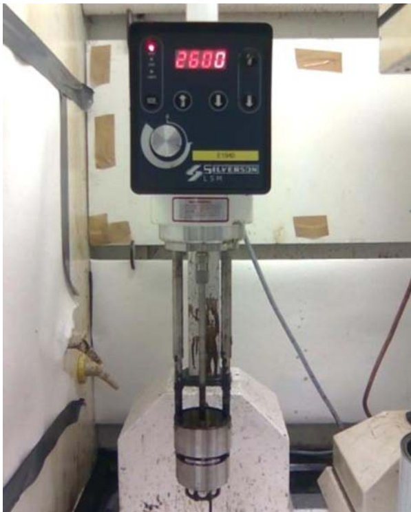
FIG. 1. HIGH SHEAR MIXER (LEFT) AND FUNCTIONAL SCHEMATIC OF THE MIXER (RIGHT)
