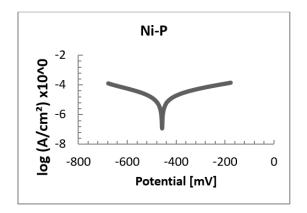
**Figure 11.** Corrosion behavior of Ni-P alloy obtained from a bath containing NiSO4.6H2O 25g/L, Sodium hypophosphite 15g/L, Am. Sulfate 15 g/L, sodium dodecyl sulfate 0.1g/L, Succinic acid 0.3g/L, Sodium gluconate 15g/L, time 60 min, pH 9, temperature 900C.
