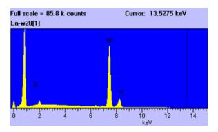
Figure 5. EDX chart of Ni91%-P3%-W6% alloy obtained from a bath containing NiSO4.6H2O 25g/L, Sodium hypophosphite 15g/L, sodium tungsten 5g/L, Am. Sulfate 15 g/L, sodium dodecyl
