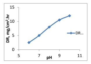
**Figure 2.** Effect of pH in the DR of Ni-P-W alloy from a bath containing NiSO4.6H2O 25g/L, Sodium hypophosphite 15g/L, sodium tungstate 15g/L, Am. Sulfate 15 g/l, sodium dodecyl sulfate 0.1g/L, Succinic acid 0.3g/L, Sodium gluconate 15g/L, time 60 min, temperature 900C.
