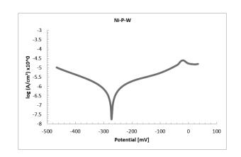
**Figure 12.** corrosion behavior of Ni94%-P2.5%-W3.5% alloy obtained from a bath containing NiSO4.6H2O 25g/L, Sodium hypophosphite 15g/L, sodium tungsten 5g/L, Am. Sulfate 15 g/L, sodium dodecyl sulfate 0.1g/L, Succinic acid 0.3g/L, Sodium gluconate 15g/L, time 60 min, pH 9, temperature 900C.
