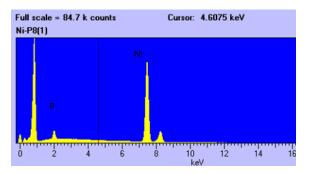
**Figure 4.** EDX chart of Ni88%-P12% alloy obtained from a bath containing NiSO4.6H2O 25g/L, Sodium hypophosphite 15g/L, Am. Sulfate 15 g/L, sodium dodecyl sulfate 0.1g/L, Succinic acid 0.3g/L, Sodium gluconate 15g/L, time 60 min, pH 9, temperature 900C.
