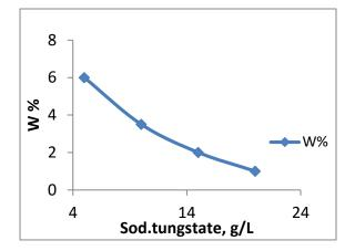
**Figure 3.** Effect of sodium tungstate g/L in W% in Ni-P-W alloy from a bath containing NiSO4.6H2O 25g/L, Sodium hypophosphite 15g/L, Am. Sulfate 15 g/L, sodium dodecyl sulfate 0.1g/L, Succinic acid 0.3g/L, Sodium gluconate 15g/L, time 60 min, pH 9, temperature 900C.
