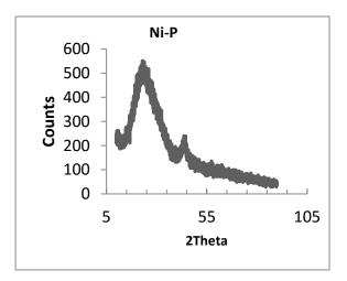
**Figure 6.** XRD chart of Ni-P alloy obtained from a bath containing NiSO4.6H2O 25g/L, Sodium hypophosphite 15g/L, Am. Sulfate 15 g/L, sodium dodecyl sulfate 0.1g/L, Succinic acid 0.3g/L, Sodium gluconate 15g/L, time 60 min, pH 9, temperature 900C.
