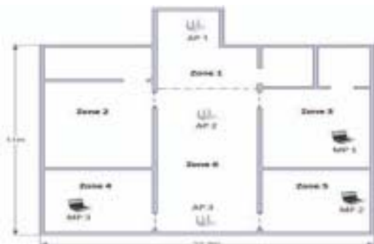
The access points (APs) represent the transmitting units while the wireless sniffers represent the Monitoring Points (MPs).
