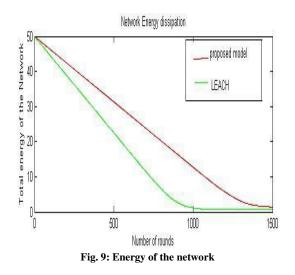
Residual energy of the network in each round gives, rate of total energy consumption, which can be a good metric to measure the energy efficiency of the algorithms. Residual energy plot is shown in fig.9.In the proposed algorithm (fig 9) the residual energy of network is much more than LEACH.
