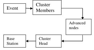
Fig. 3: Data propagation in WSN
