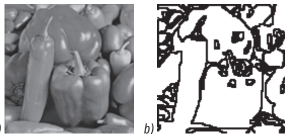
Fig. 4. Resulted algorithm performance for the image "Peppers": a) the original image, b) the contours resulting from the 4th level clustering
