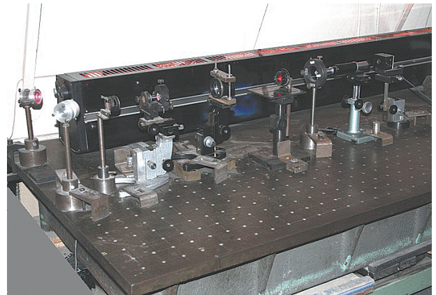
Fig. 3. Pilot unit assembled on the "SYN"-type interferometer table and enabled to transfer the formed picture to computer for analysis
