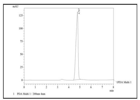
Fig. 2: Chromatrogram of VLB under optimized mobile phase condition[Acetonitrile: Water (20: 80, % v/v)]
