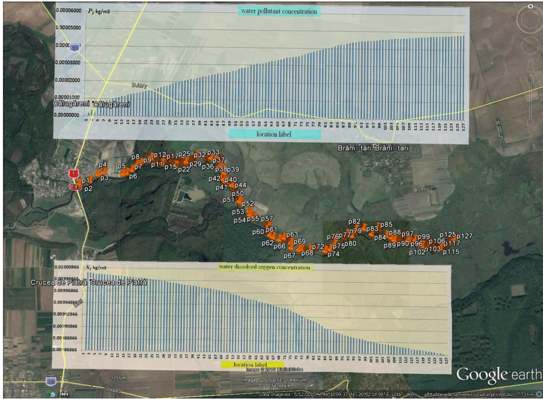
Fig.1 - Variation in pollutant and water dissolved oxygen concentrations along a section of river
