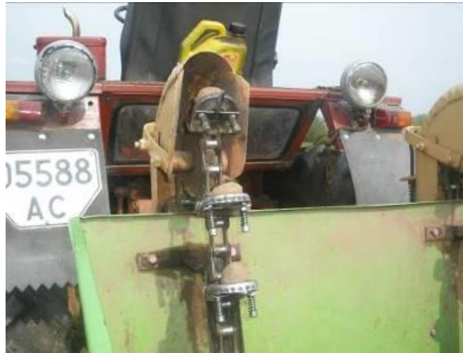
Fig.4 – Tractor with potato-planter with apparatus with spring needle
