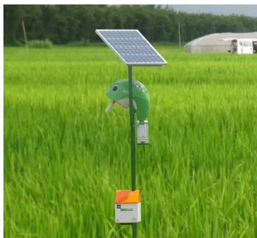
Fig.1 - Acquisition system of rice planthopper images
