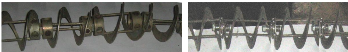
Fig.9 - Sectional screw operating members with a) hinged joints; b) safety joints
