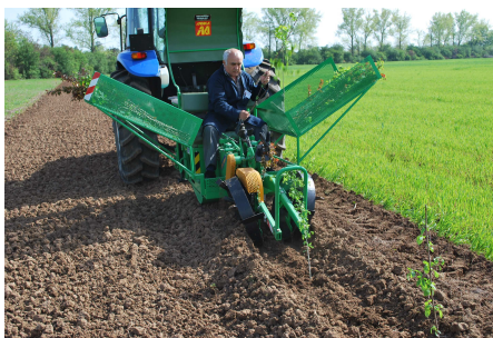
Fig. 5- Equipment of planting forestry seedlings, EPF1 / Echipament de plantat puieti forestier--EPF1-în lucru
