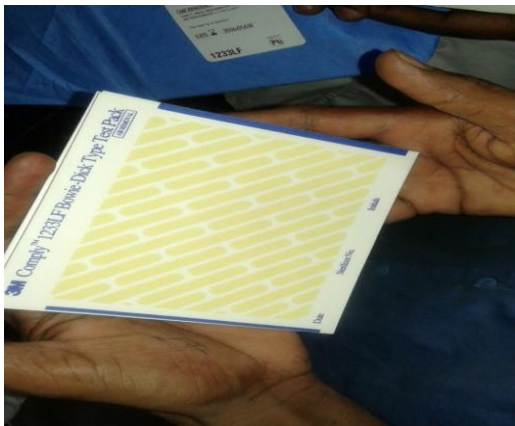
Figure 14: Bowie Dick test paper (Before sterilization)
