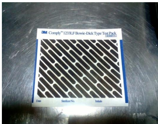
Figure 15: Bowie Dick test paper (After sterilization)
