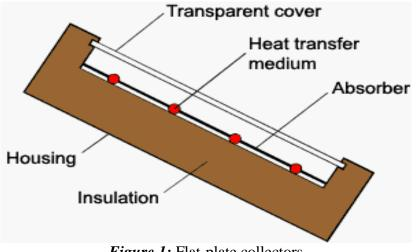
*Figure 1:* Flat-plate collectors
