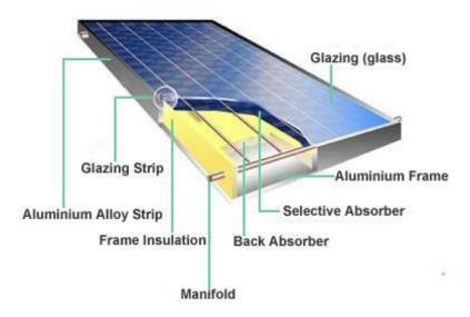
Figure 2: Flat-plate collectors with absorbers
