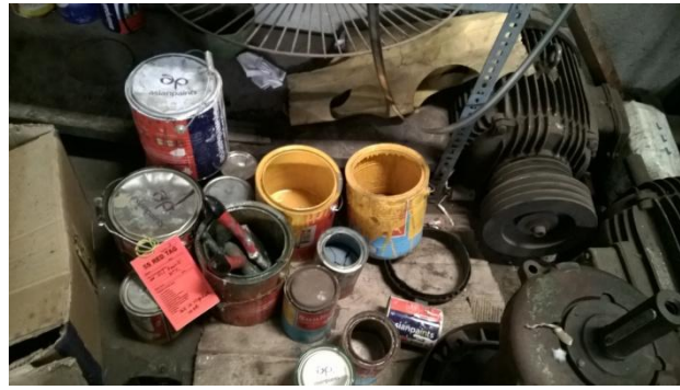
Fig 9 Red tagging to unwanted material
