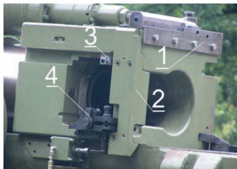
Figure 12 – Breech ring, left lateral view
