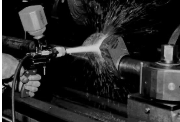
Slika 4 – Nanošenje prevlake na rukavac kolenastog vratila plazma pištoljem Figure 4 – Coating deposition on a crankshaft pin by the plasma gun
