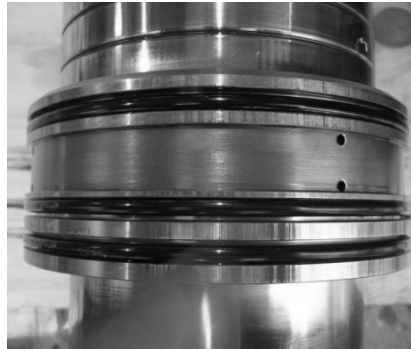
Figure 11 – Abrasive damage of the regulating valve piston Slika 11 – Abrazivna oštećenja na klipu regulacionog ventila
