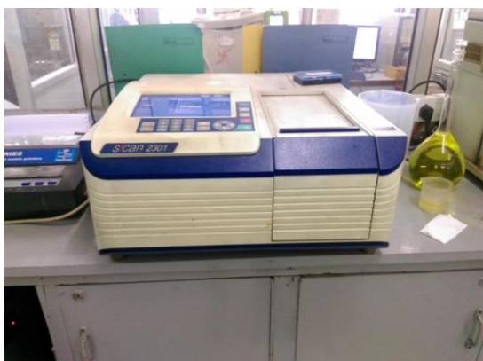
Fig 2: SCAIN-2301 double beam Ultraviolet spectrophotometer
