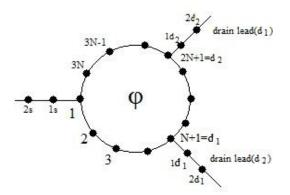
Fig. 1: A schematic view of a three-terminal semiconductor mesoscopic ring
