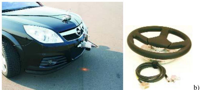
Figure 11 MSW/S - Measurement Steering Wheel for non-contact measurement of steering speed and angle
