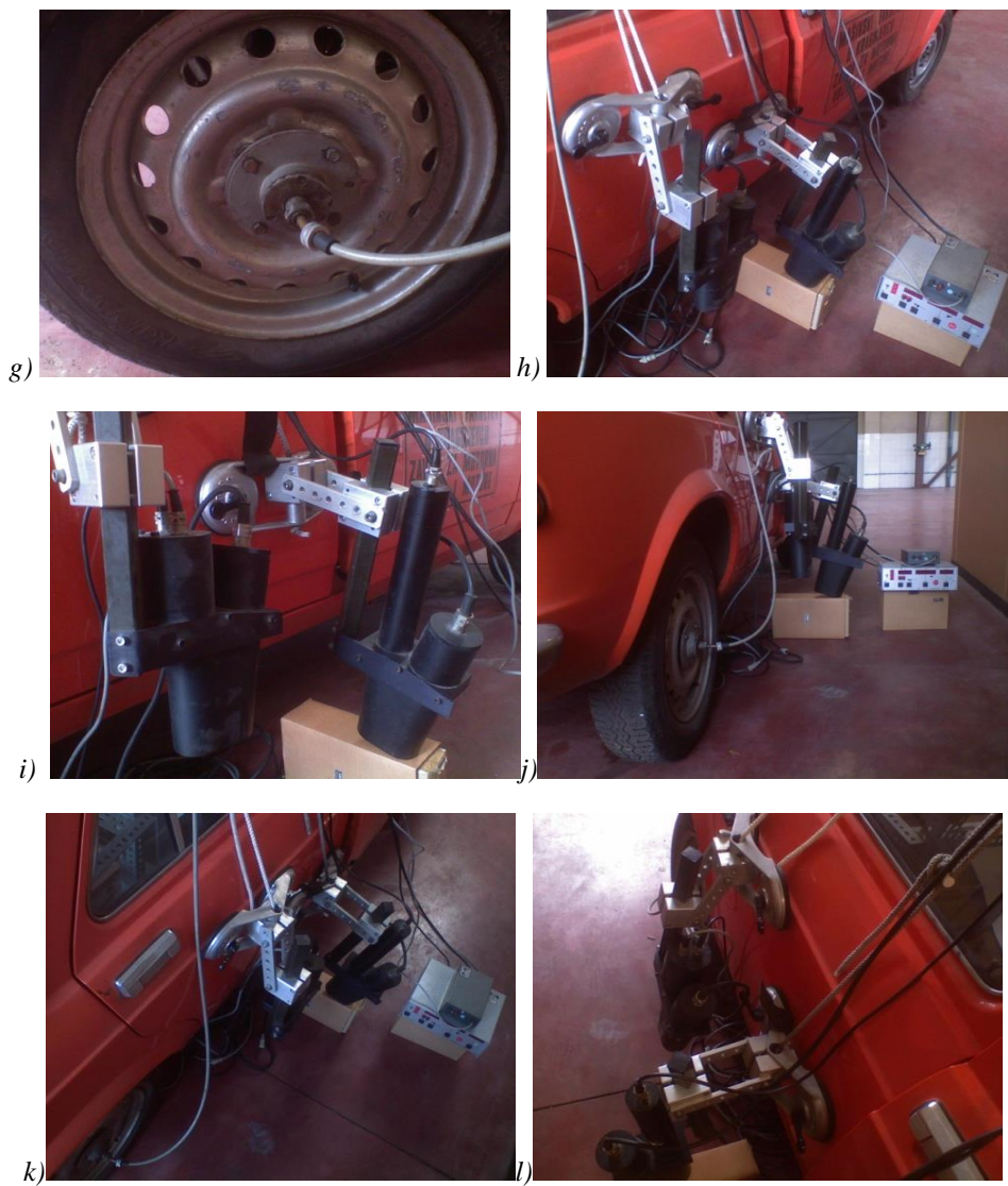
Figure 13 Sensors for Motor Vehicle Measurement: a), c) steering wheel speed, angle and torque, b) brake pressure HBM, d), e), f), h), i), j), k), l), vehicle lateral and longitudinal velocity Leitz – Correvit, L -, Q- Sensors, d), g) wheel angular velocity, own design.
