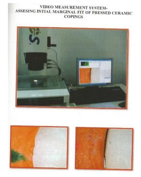
marginal fit of the coping. The measurement sites were marked for reproducible identification by scoring the die with sharp blade.
