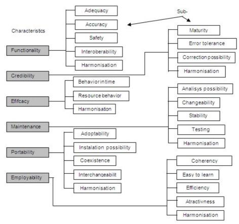
Figure 6. Software evaluation with internal and external aspects
