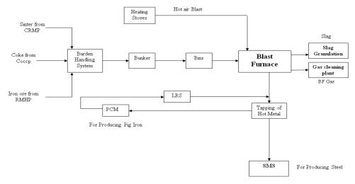
Figure 1. Process flow diagram of Hot Metal process in Blast Furnace
