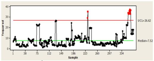
Figure 10. T<sup>2</sup> Generalized variance chart for critical process variables
