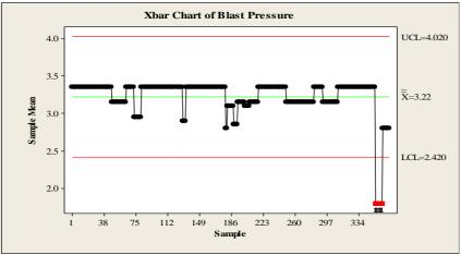
Figure 2.  $\overline{X}$ Chart of Blast Pressure
