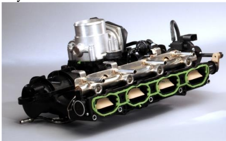
Figure 3. Air Intake Manifold
