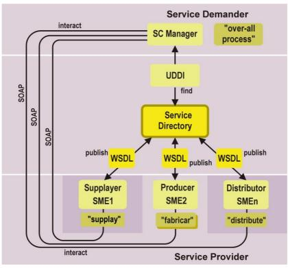
Figure 4. Architecture of supply chain management systems using SOA
