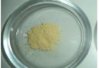
Fig. 2: ZnO nanoparticles synthesized from Calotropis procera
