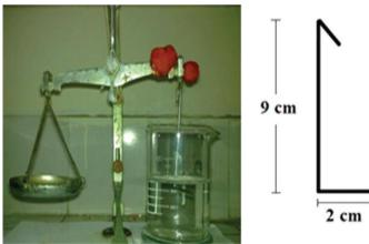
Fig. 1: (a) Modified balance method (b) Wire probe for raft strength measurement
