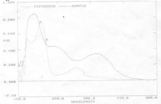
Fig. 3: UV overlain absorption plot of Desvenlafaxine and Clonazepam
