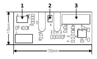
Fig. 5. Schematic of the separated sensor board with separated sensors on it. 1: MPL3115A2 barometer. 2: MCP9808 thermometer. 3: HIH-5031 relative humidity sensor.
