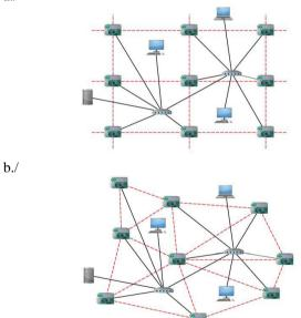
Fig. 1. The conception of DSN-PC sensor network, which forms the necessary grid for numerical calculations by using the nodes of the networked sensor stations not only for measurements and collection of data but for communication with their close and distant neighbors through the Internet and solve numerical weather prediction calculations by the Finite Difference Method (FDM) on a rectangular grid (a./) or by the Finite Elements Method (FEM) on irregular grid (b./) [2].
