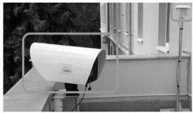
Fig. 1. Free Space Optics head (model Light Point – Flight Strata 155) on the left. Fog sensor with ability of measuring different atmosphere paramteres (temperature, humidity, preassure, altitude, lwc). This setup is located within a campus of Technical University of Kosice (Vysokoskolska 4).
