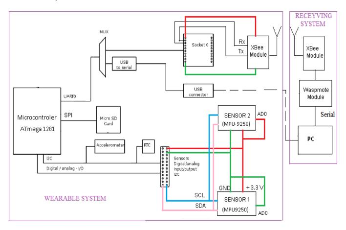
Fig.1. Data acquisition system using two inertial sensors
