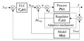
Figure 5. Behavior model control (functional diagram).
