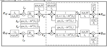
Figure 1. Power control of DFIG.
