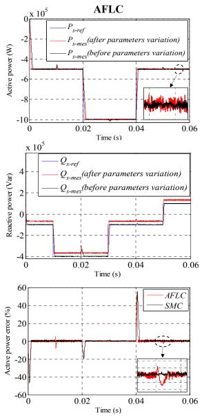
Figure 9. Effect of machine's parameters variation on the DFIG control.
