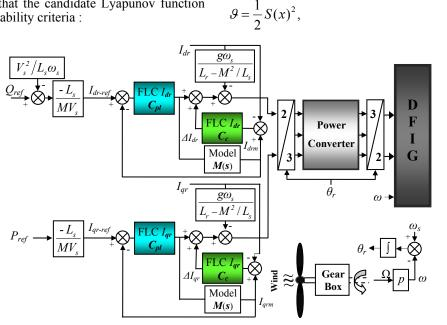
Figure 6. Bloc diagram of the adaptive fuzzy logic control of the DFIG.
