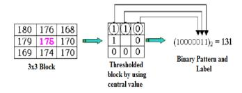
Fig 4. Illustration of Local Binary Pattern Calculation
