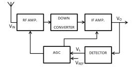
Fig. 1. Analog frontend of a generic radioreceiver.
