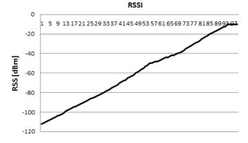
Fig. 4. RSS as a function of RSSI for Cisco routers
