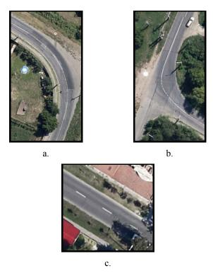
Fig. 3. Example of segment types: a. sag curve, b. crest curve, c. plain segment [25]
