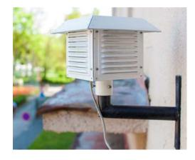
Fig. 3. Fog sensor device.
