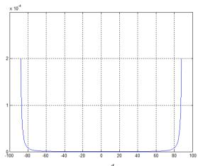
Fig. 2.  $CRB_{ULA}$  for K = 1, SNR = 20 dB,  $\frac{d}{2} = 0.5$ , M = 16, f = 2.4 GHz
