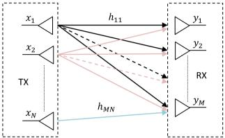
Fig. 1. NxM MIMO channel matrix - complex coefficients  $h_{ji}$ .
